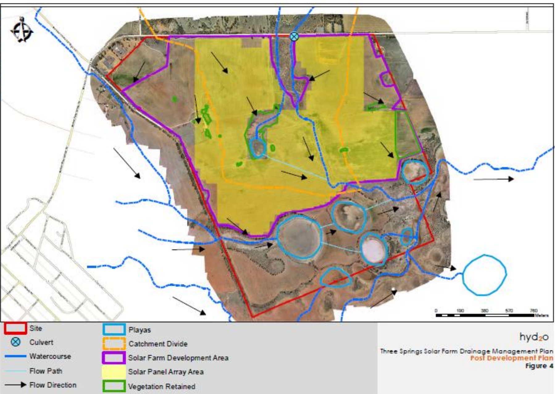
FIGURE 4 – POST DEVELOPMENT DRAINAGE
