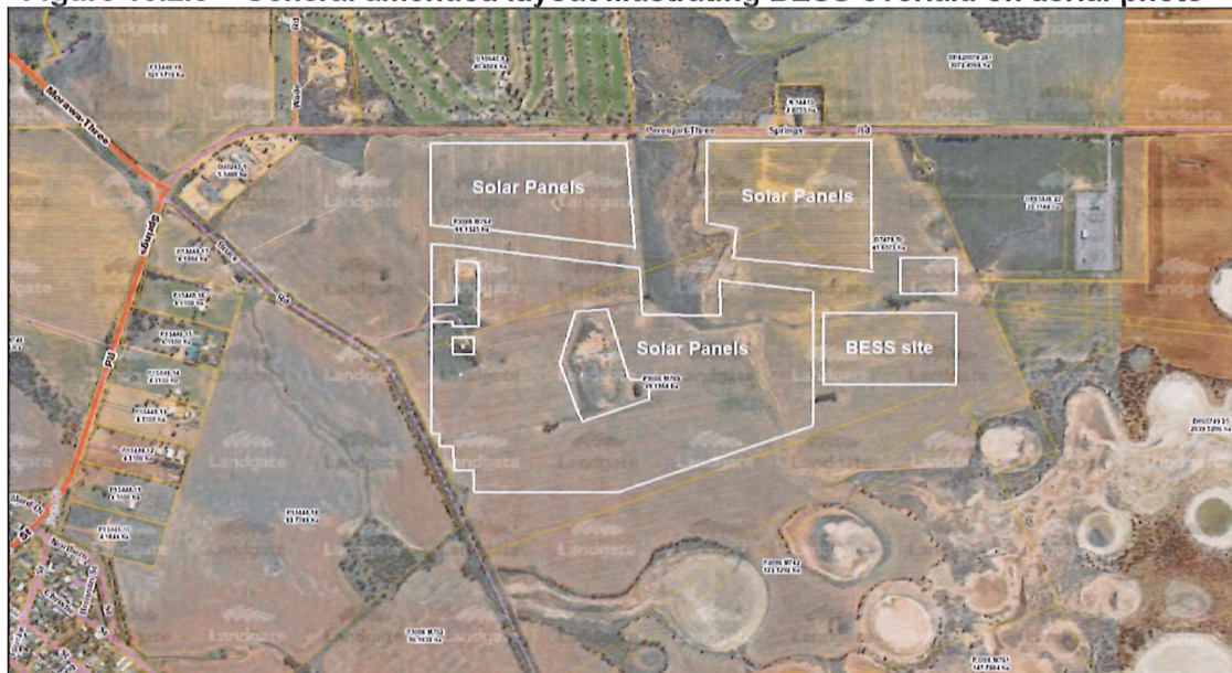
Figure 10.2.6 – General amended layout illustrating BESS overlaid on aerial photo
